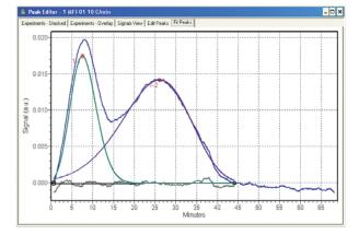
In addition to standard peak integration, peak fitting is also included to allow effective separation and modeling of convolved signals.
