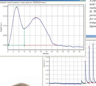
A full-feature peak editor and integration package is included with the AutoChem II. This easy-to-use package provides a rapid method for evaluating common temperature-programmed and dynamic adsorption data.
