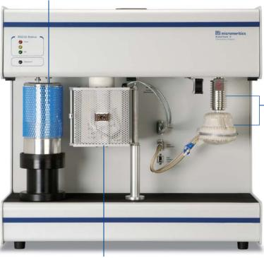
Vapor Generator featuring two zones to ensure a saturated vapor is produced
