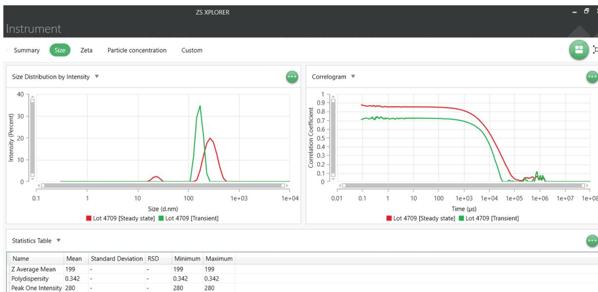
ZS Xplorer features a new algorithm called Adaptive Correlation that uses information from the sample to determine how long it should be measured for, collecting data until the final answer has become consistent. This feature also applies intelligent logic to separate erroneous data associated with transient artefacts such as dust or aggregates, which may previously have required diagnosis by an experienced user followed by additional sample preparation.
