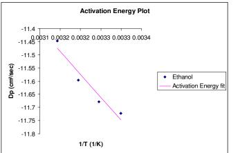
A, B and C are constants describing different diffusion regimes. C represents all non-equilibrium properties and is therefore directly related to the bulk diffusion constant. In the actual example [11], the diffusion of ethanol and octane into an anti-obesity drug was measured. The diffusion coefficient for ethanol yields to  $8.12*10^{-6}$  while octane gives  $4.12*10^{-5}$  cm<sup>2</sup>/sec (for a particle size of
