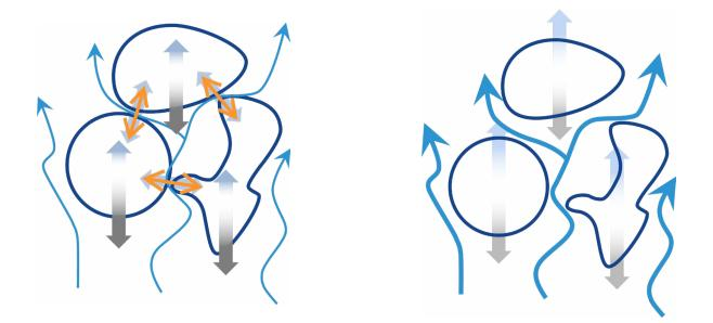
If cohesive forces are very large, air drag must be significantly higher to achieve fluidization. In some cases, where  $F_{coh}/W$  >> 1, most particles remain in contact with one another; high air speeds separate some particles and form a small number of channels through the powder bed. These channels divert the applied air flow and the powder does not achieve fluidization at all.
