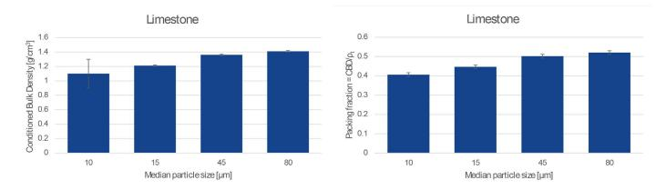
When comparing powders with similar skeletal density, and similar particle size distribution span, a higher cohesivity (higher  $F_{coh}/W$  value) manifests as a lower Conditioned Bulk Density. Moreover, if the skeletal density is known (see Accupyc), the fraction of the bulk volume occupied by solid particles can be found. The solid volume fraction indicates particle packing efficiency and it is higher the lower the cohesivity of the powder.
