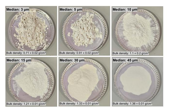
With larger particle size, the surface of the powder heaps becomes noticeably smoother, with visibly less clumps, and we also measured the bulk density to increase as particles arrange more efficiently under gravity.
