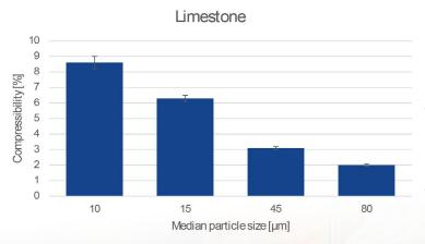
Measuring the difference in volume between the gravitationally-packed and compressed states provides a value for the powder Compressibility. As more cohesive powders tend to contain a larger proportion of empty spaces between particles, the bulk contains more space for particles to rearrange into when a comparatively large external load compresses the powder. a micromeritics' company
