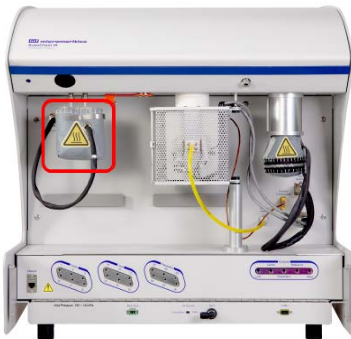
Heating mantle shown installed
