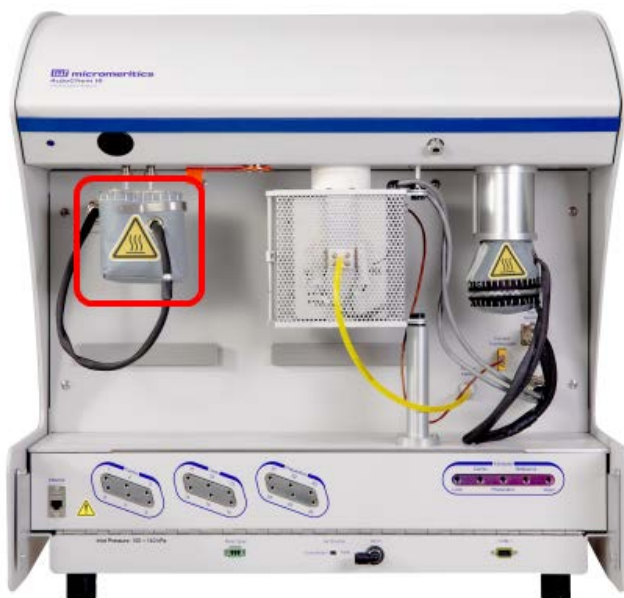
Sorption trap inside heating mantle
